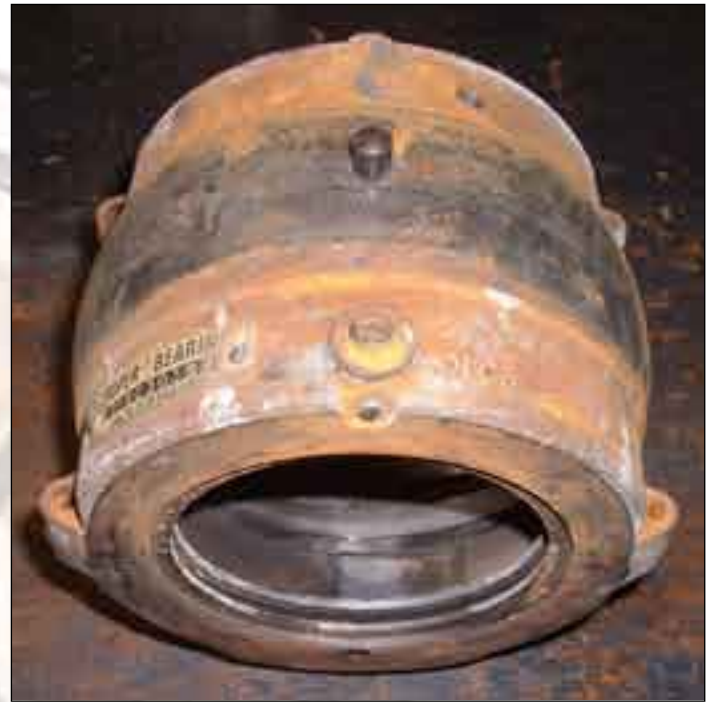
This Cooper 01C408GR is typical of many of the bearings Cooper receives for refurbishment. A full assessment is carried out before work is started.
